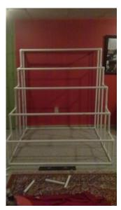
Complete the remaining steps similar to the second step. The last step (5th step) uses 9" pipe.
