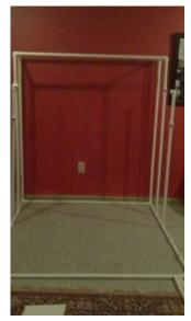
Install two 35" pipes onto the next two tees. Insert two tees on top and attach 9" pipes on top of each tee.
