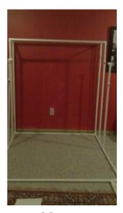
Install two 35" pipes onto the next two tees. Insert two tees on top and attach 9" pipes on top of each tee.
